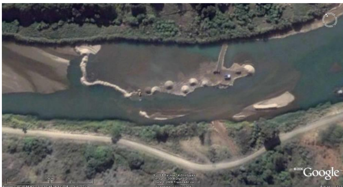
Figure 5.2: Example of sand mining operations directly in uMkhomazi main river channel (Aerial view generated from Google Earth™ 2008©)
